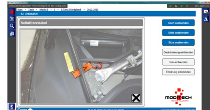
Graphics to components and safety systems
