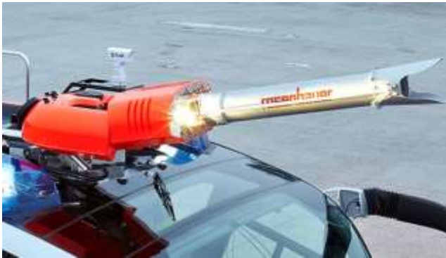
Turret with foam barrel and deflector
