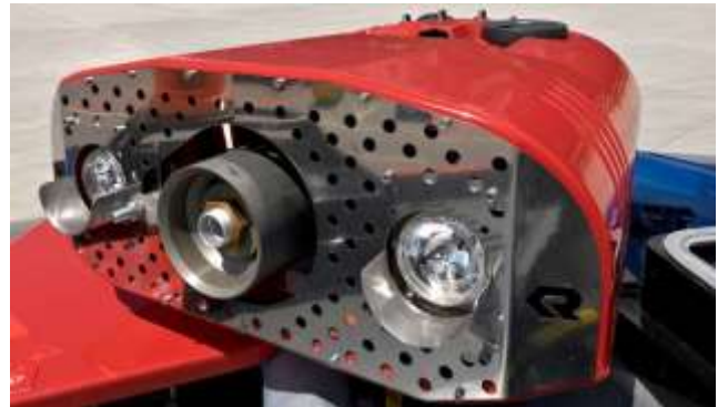
Turret with ChemCore nozzle
