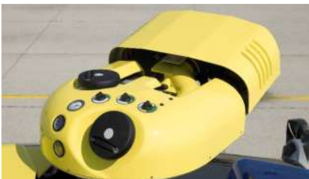
Manual emergency actuation on turret
