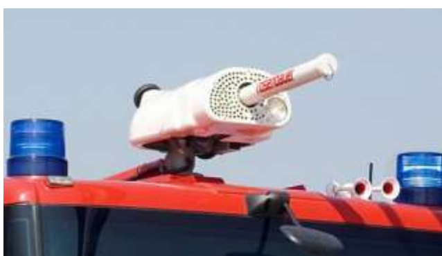
Dry chemical turret
