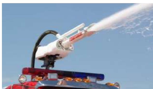
Turret with foam barrel and deflector, top mounted dry chem nozzle
