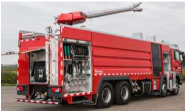
Turret with foam barrel and deflector
