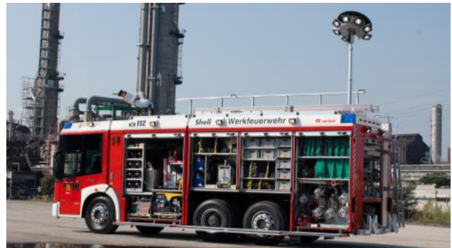
Industry fire fighting truck with direct injection foam system HYDROMATIC and R600
