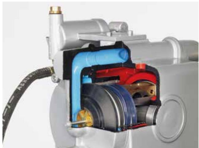
Piston priming pump with automatic priming - mounted above the centrifugal pump
