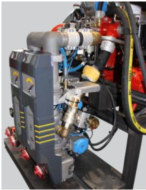
Modular CAFS piping
