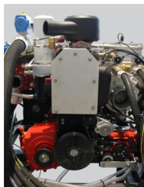
Integrated and on and off switchable compressor
